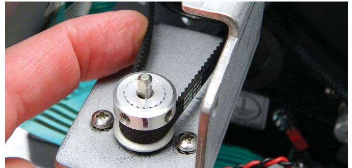
Step 12: After all 3 screws have been tightened, press on the belt to make sure that the tension seems good. The photo shows the correct amount of tension.
