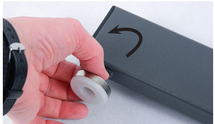
Step 4: Remove four stand levelers (if installed) by rotating counter clockwise (CCW). Use a 7/16" wrench to loosen if the levers if they are tight.
