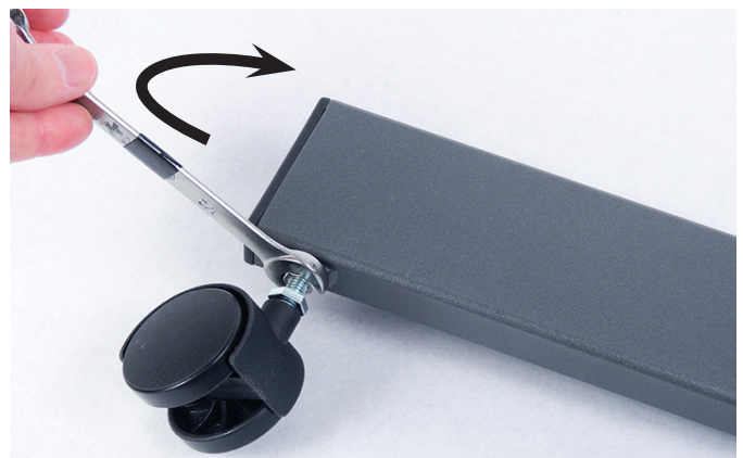
Step 6: Tighten the nut clockwise with the 1/2" wrench to lock in place. Hold the caster still with the 9/16" wrench if needed. Repeat steps 1-6 with the other 3 wheels. NOTE: Level the machine following the directions in the user guide after all wheels are installed. ...FINISHED
