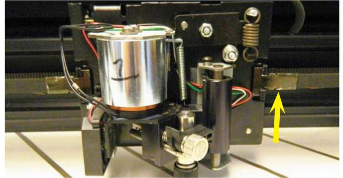
Step 8: (**300-350HF**) Hold carriage with the LEFT hand and pull the belt (yellow arrow) toward the carriage to remove it. Repeat on other side making sure not to tangle in wires. **NOTE: Do not remove the carriage.**
