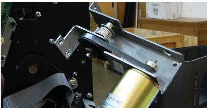
Step 11: Remove the old Y transmission and place to the side.
