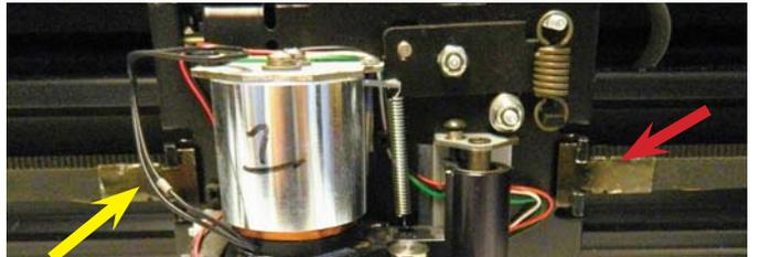
Step 17: (**300-350HF**) Align the Y belt in the tensioner then get the belt ends near the carriage. Hook the tensioner end of the belt (yellow arrow) onto the carriage then hold the carriage while pulling the keypad end of the belt to hook it into the right side of the carriage (red arrow).
