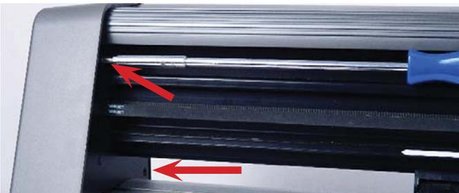
Step 5: Remove the left end cover by unscrewing the (2) screws (red arrows). This will give you access to the carriage (Y) belt tensioner.
