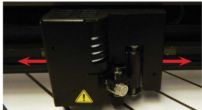
Step 7: (**300/350HF**): Remove the **carriage cover** by gently pulling the edges (red arrows) of the cover away from base then rotating up.
