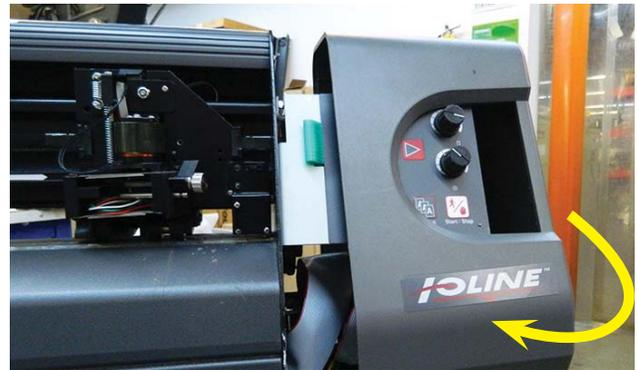
Step 4: Pull the right cover away from machine then rotate it toward the front of the machine to avoid the keypad adjustment knobs.
