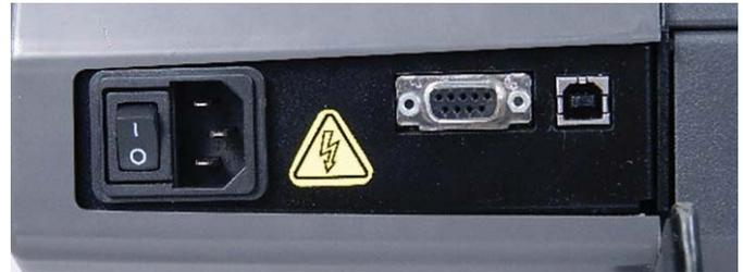
Step 2: Turn off, then unplug the power cord and the communication cable.
