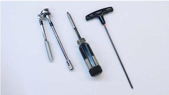
Step 1: Tools needed: An 11/32" socket wrench & 6" extension, Phillips screwdriver and 9/64" hex wrench.
