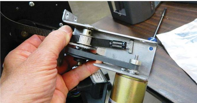
Step 13: Before placing the new Y transmission on the machine, thread the Y belt behind and around the pulley.
